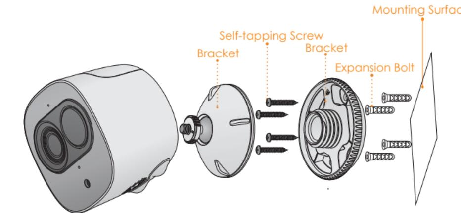
**Step1** Drill screw holes on the mounting surface as the positioning map shows, and then put in the expansion bolts.
