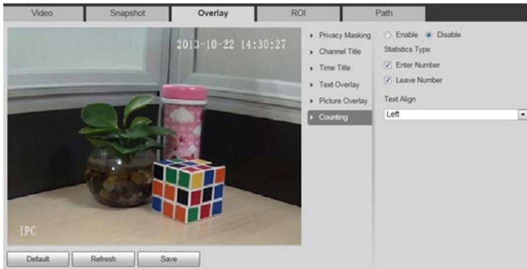
**Step 2** Select the **Enable** checkbox, and then configure counting method and alignment.
