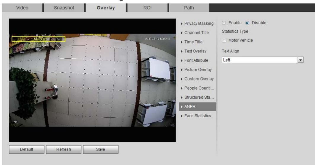
**Step 2** Select the **Enable** checkbox, select the statistics type, and then select text align.
