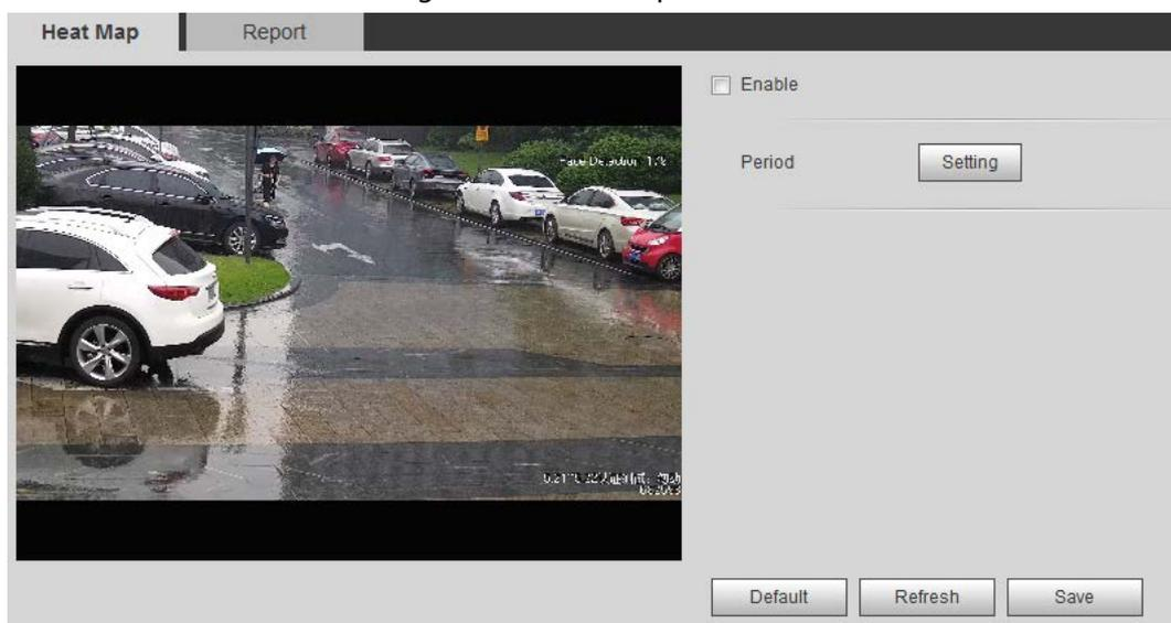
Step 2 Select the **Enable** checkbox to enable the heat map function.
