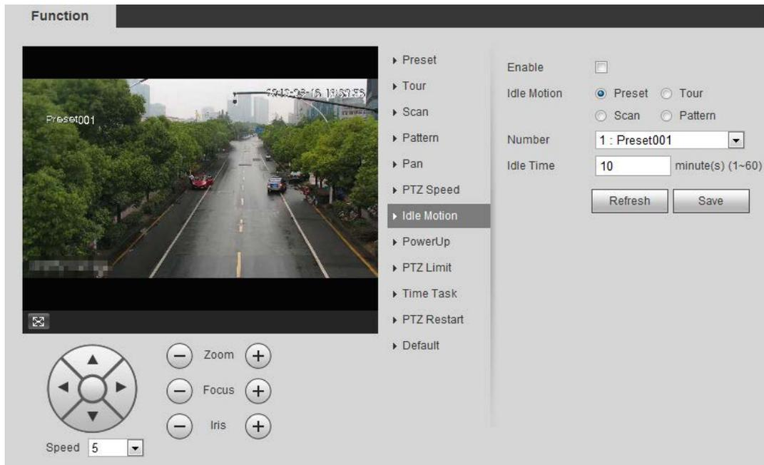
**Step 2** Select the **Enable** checkbox to enable the idle motion function.
