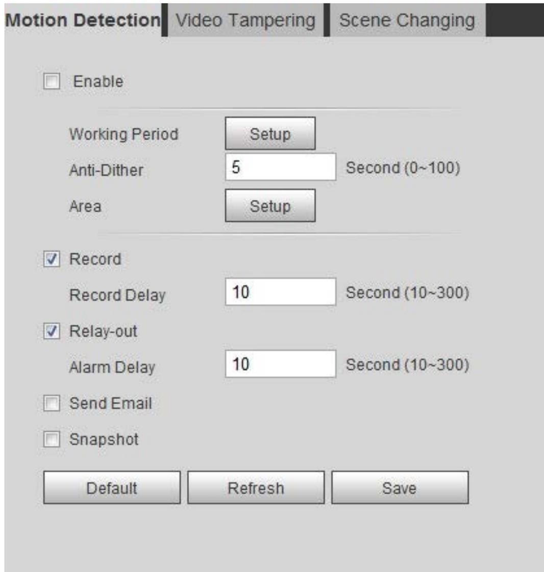
Step 2 Select the **Enable** checkbox to enable motion detection function.
