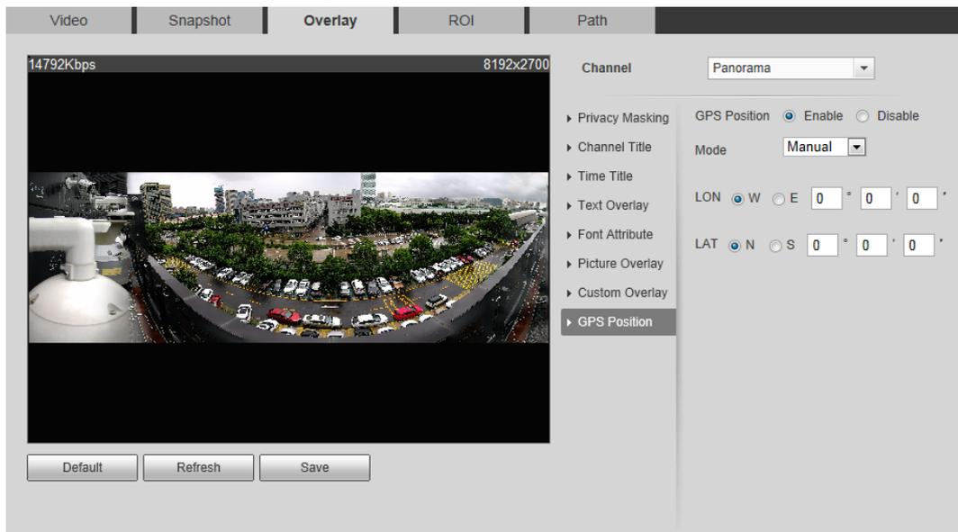
Step 2 Select the **Enable** checkbox, and then select the **Mode** to **Auto** or **Manual**.
