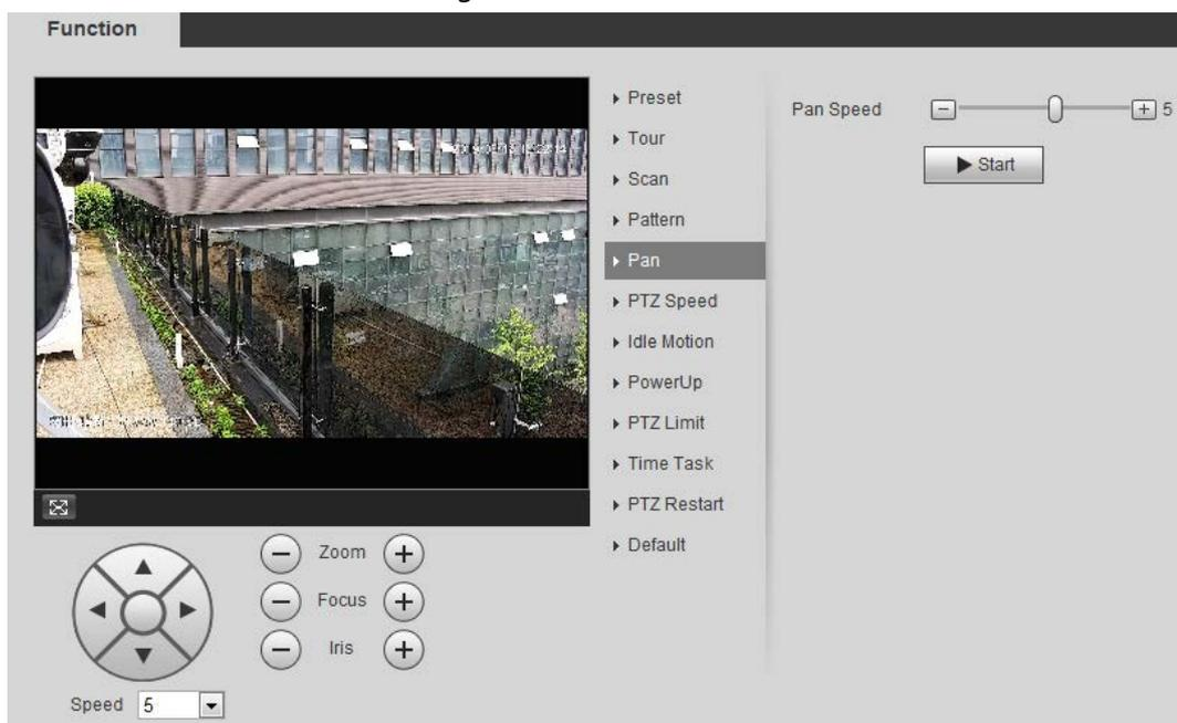
Step 2 Set the pan speed and click **Start**, and the camera starts horizontal rotation.
