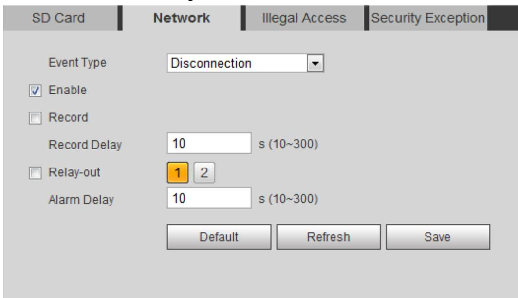
**Step 2** Select the event type from the **Event Type** drop-down list, and then select the **Enable** checkbox to enable the network detection function.
