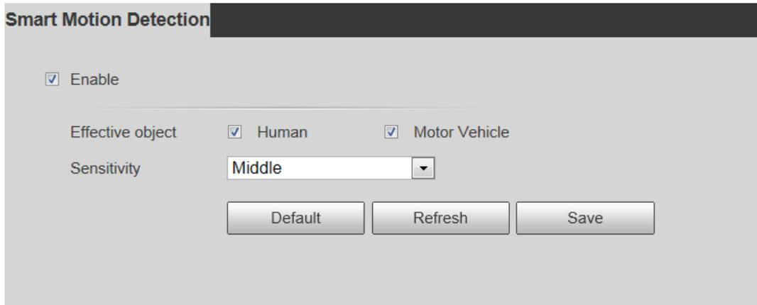
Step 2 Select the **Enable** checkbox to enable the smart motion detection function.
