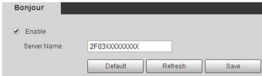
**Step 2** Select the **Enable** checkbox, and then configure server name.
