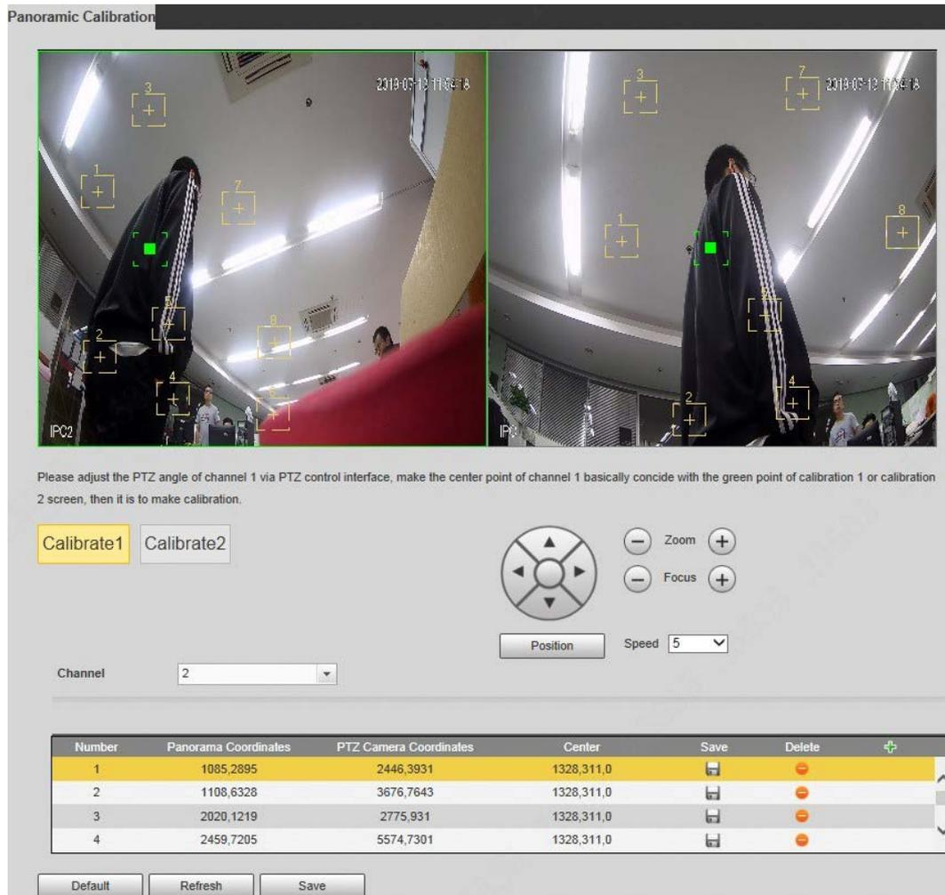
**Step 2** Select channel 2, and then select a calibration number under the video images in turns (See Figure 5-21) to add calibration points to the corresponding video images. Take **Calibrate 1** as an example.
