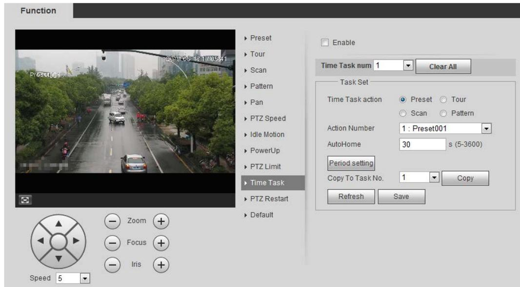
**Step 2** Select the **Enable** checkbox to enable time task function.
