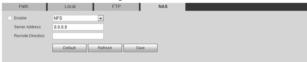
Step 2 Select the **Enable** checkbox to enable NAS function, and select NAS protocol type.
