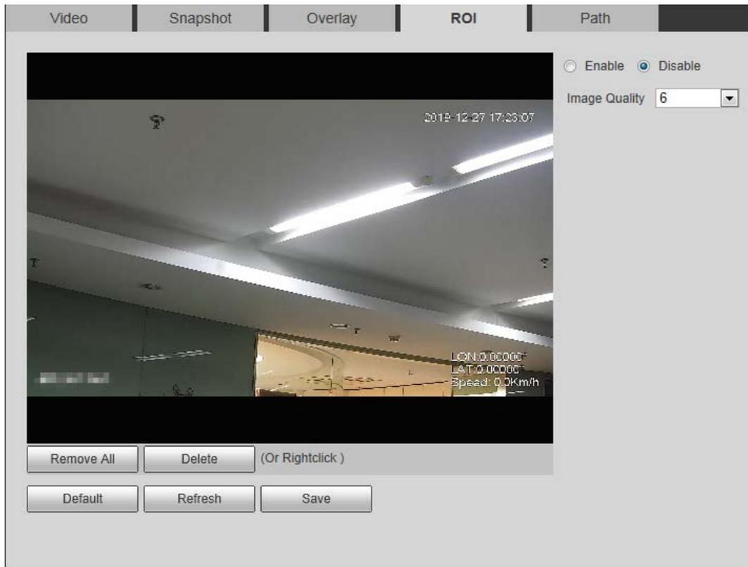
**Step 2** Select the **Enable** checkbox, draw the area on the image, and then configure the image quality of ROI.
