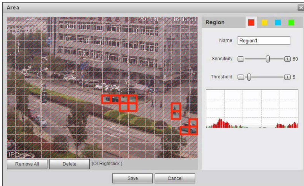
2) Select a color and set the region name. Select an effective area for Motion Detection in the image and set **Sensitivity** and **Threshold**.
