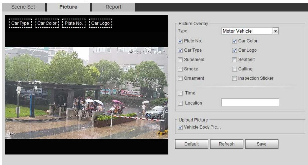
**Step 2** Select **Motor Vehicle** from the **Type** drop-down list.
